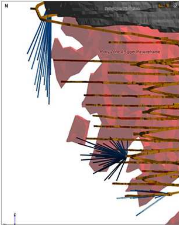
FIGURE 3: Longitudinal view, looking east, of the currently defined limits to the Roby Zone (red solid) showing location of the fall 2012 extension drilling program and the underground ramp system.
